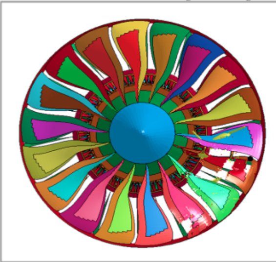
Figure IV.6 Blade damage following drone ingestion. After the drone cleared the fan stage of the engine in the simulation, three engine blades had failed.
